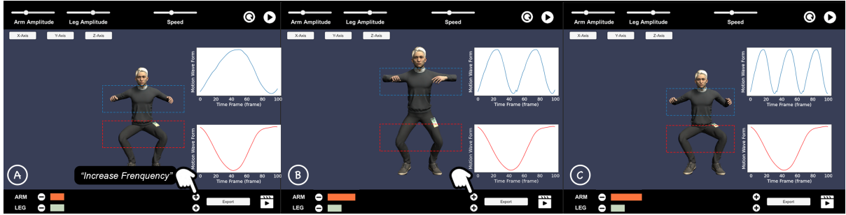
Fig. 8. Motion combination function. A single upper-body motion (raise hand) can be added to a single lower-body motion (squatting). Pressing the plus button will increase the frequency of the upper-limb motion (e.g., to three). This means that the lower limbs perform one movement, while the upper limbs perform three movements.
